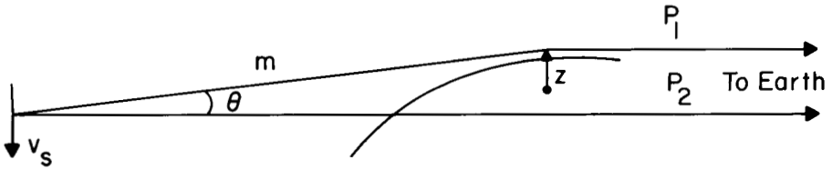
Fig. 4. Occultation geometry for a radio experiment at immersion. The velocity v_s is the component in the plane of the figure and at right angles to path P_2 of the actual spacecraft velocity.
