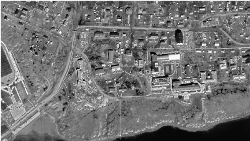
Figure 41b Aerial view of the planned sports complex showing thermokarst development. Photo credit: A. N. Fedorov.
