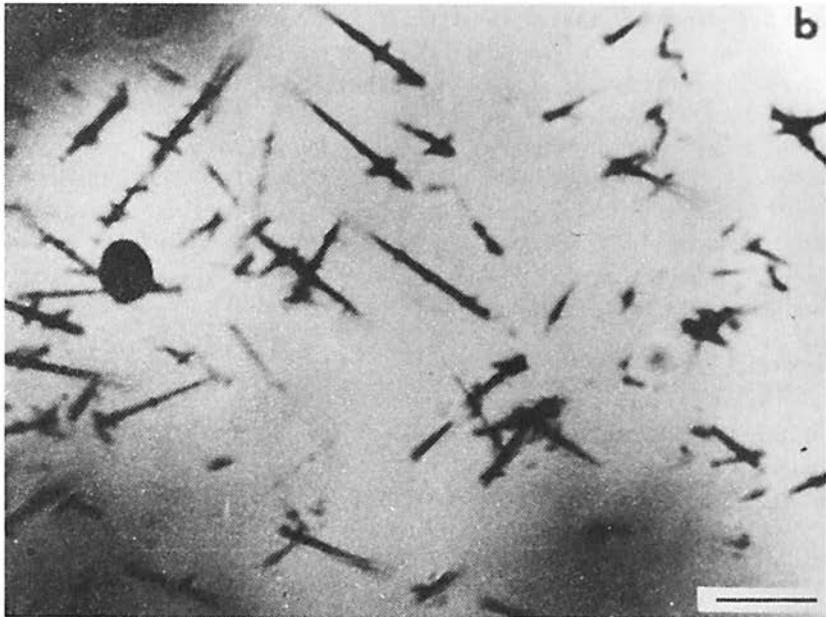
Fig. 4.1.3. (a) Tracks produced by solar-flare heavy ions. (b) Tracks produced by galactic-cosmic-ray heavy ions. These tracks become visible by optical microscopy after chemical etching. Scale bars = 1\ \mu\text{m} .
